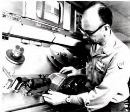
KBTV's long-life Alfecon II headwheel.
