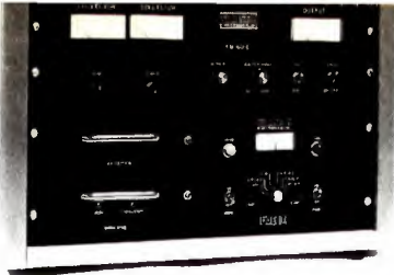
Heart of any FM transmitter is the exciter. Pictured above is one of the latest to be designed, the FME 10 (lower chassis) coupled with a 60W amplifier to make up an all solid-state FM transmitter. Unit is from Wilkinson.
