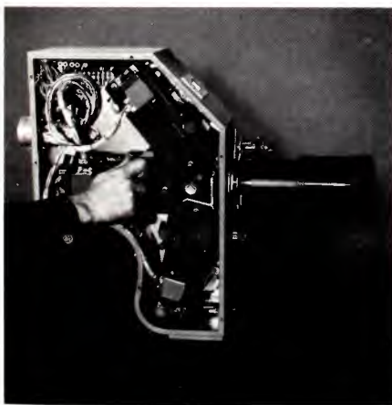
Camera-head design permits optics to be adjusted while camera is carried.
